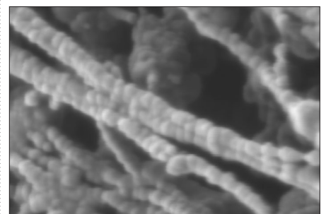
Figure 12. All catalyst particles are located at the interface of the electron conductor (carbon black) and the proton conductor (Nafion™).
