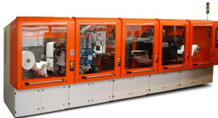
Modular roll-to-roll deposition production line microFLEX at Fraunhofer ENAS for industrial applications.
